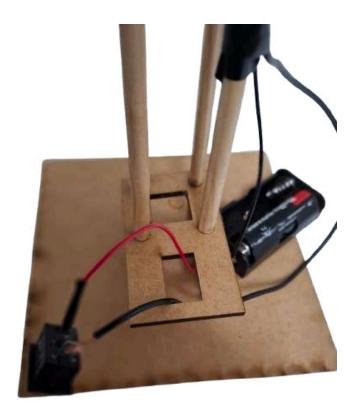
Connect the wires insert the switch in the hole provided. Connect the batteries correctly to positive and negative fitting. When you switch the switch on it should transform the wire nail a magnet. Turn the lever to draw the wire nail upward. If the magnet is not working properly please make sure the exposed wires are making contact with the switch connectors.
