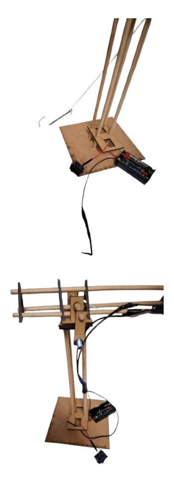
Connect one end of the wire to the switch (make sure the wire goes through the switch hole from underneath before connecting the wire to the switch.) Wind the wire tightly and in a neat fashion
